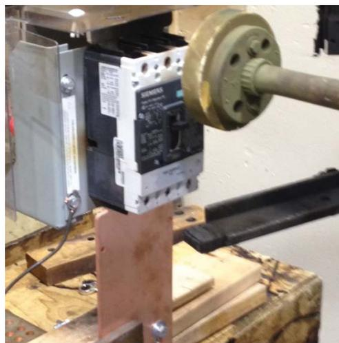
**FIGURE 4 – Arc Flash Test Set-Up**
