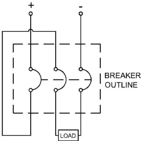
FIGURE 1 – Typical DC Breaker Wiring
