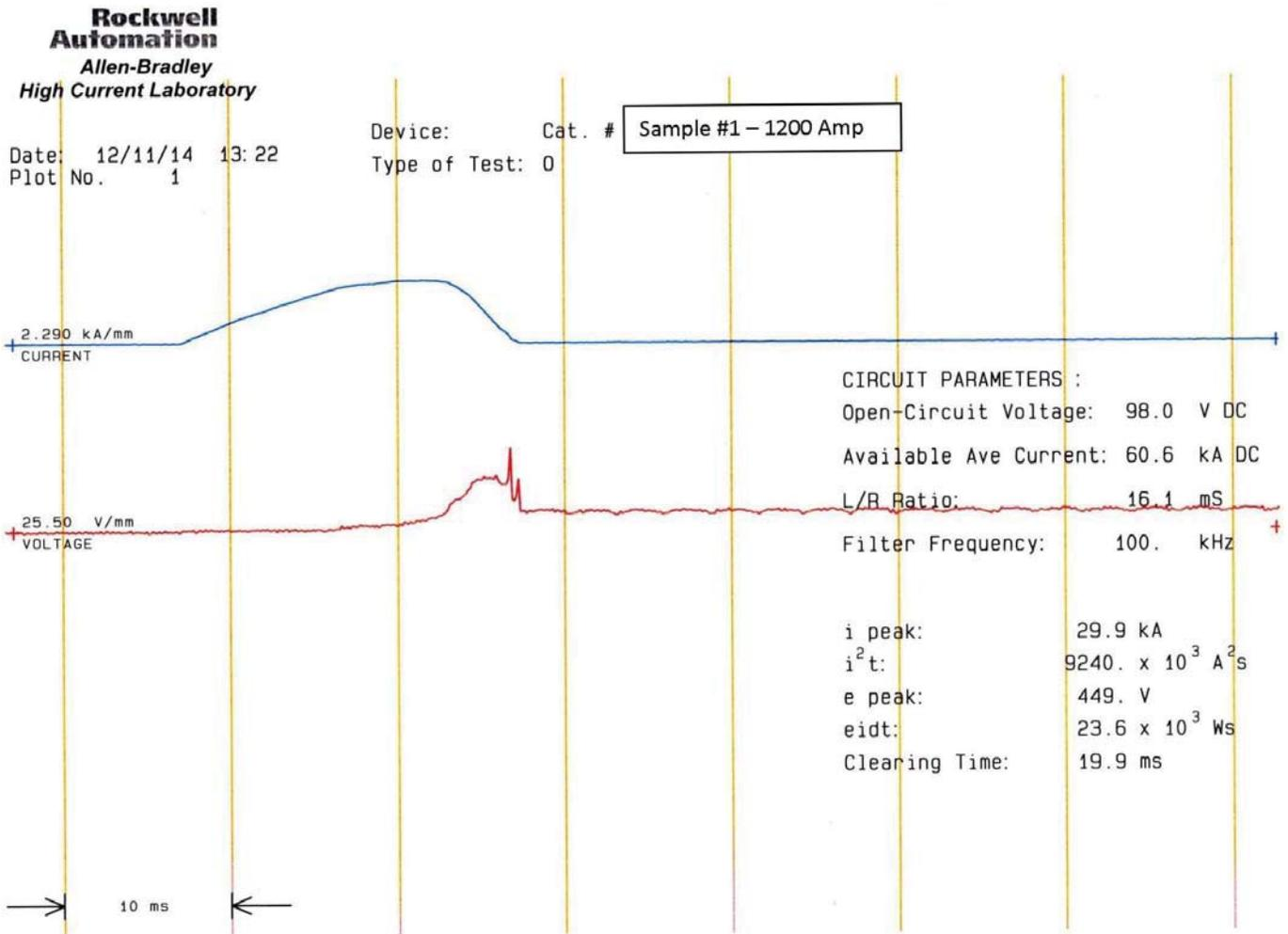
**FIGURE 5 – Short Circuit Curve (1200 Amp Sample)**
